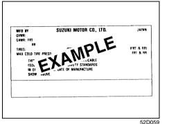
This label contains important safetyrelated information about your vehicle. The label is located on the driver's door lock pillar. Emission Compliance Label (for U.S.A.)
